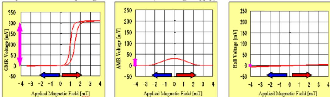
MR sensor detects horizontal magnetic field against magnet location. Hall sensor detects vertical magnetic field. In general, horizontal magnetic field has wider distribution than vertical one. So MR sensor has wider detection area than Hall sensor with same magnet size. This means MR sensor allows bigger gap between sensor vs. magnet position.
