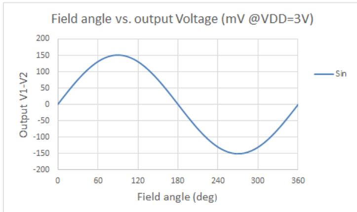
HGAR can detect 360deg magnetic field angle.
