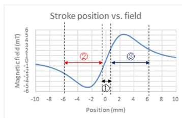
① Narrow area detection (Sensor OFF+OFF)
