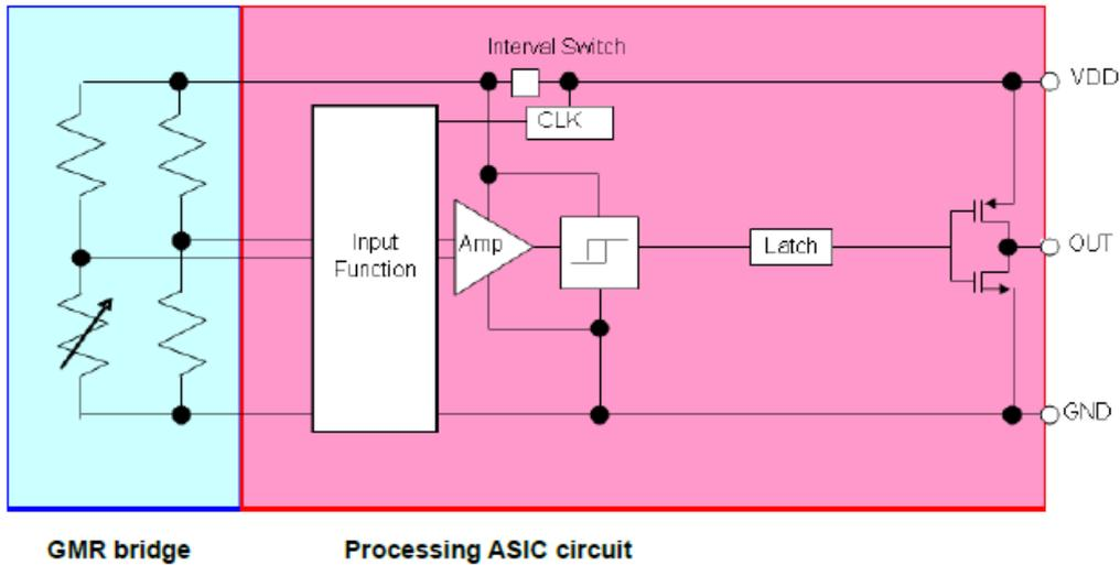
Switching HGD types can detect horizontal magnetic field, and have 3 types of function mode.
