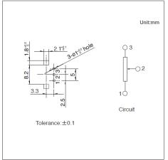
■ Terminal Layout / Circuit Diagram
