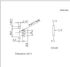
■ Terminal Layout / Circuit Diagram
