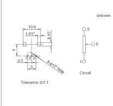
■ Terminal Layout / Circuit Diagram
