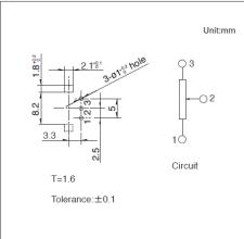
■ Terminal Layout / Circuit Diagram
