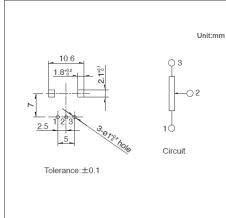
■ Terminal Layout / Circuit Diagram
