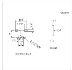
■ Terminal Layout / Circuit Diagram
