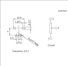
■ Terminal Layout / Circuit Diagram
