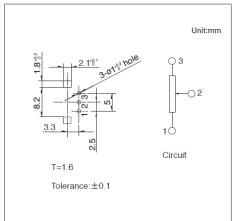
■ Terminal Layout / Circuit Diagram
