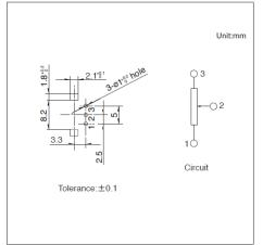
■ Terminal Layout / Circuit Diagram
